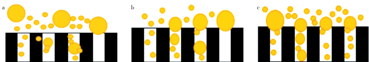
图3 膜孔堵塞示意图:(a)初始阶段;(b)过滤过程中;(c)膜孔完全堵塞 Fig. 3 Schematic diagrams of different membranes fouling:(a)Initial stage;(b)During filtration; (c)Complete blockage of membrane holes
